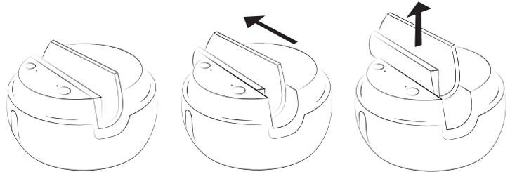
Finally, insert shim into grip holder and place in base.
