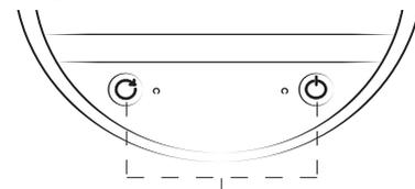
**Step 1:** Press and hold both power and sync button simultaneously until power LED on base flashes. Then release.
